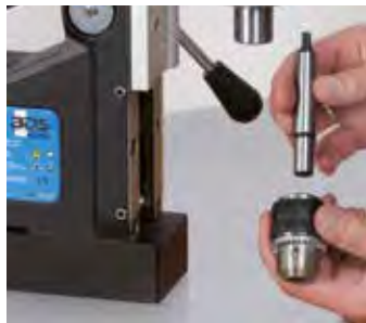
1. Connect taper drift to drill chuck.
