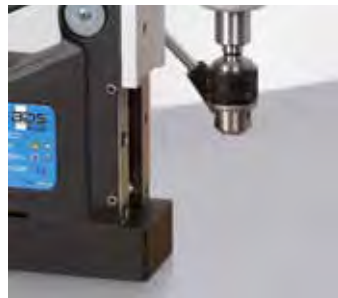
2. Insert drill chuck in MT arbor.
