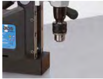
2. Insert drill chuck into the direct arbor.
