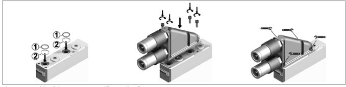
Fig. 13: Assembly of the customer-specific coupling flange
