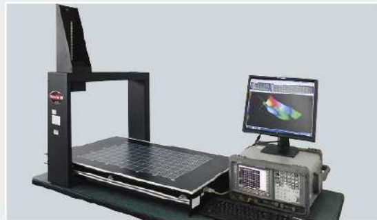
Whole set of EMI scanner (Detectus AB company, Sweden) & Anti-interference developing system (Agilent company, USA)
