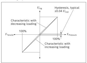
▼ Characteristic curve 2 (load range from 60 kN)
