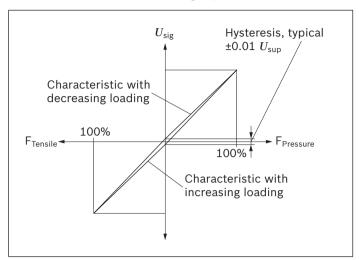
▼ Characteristic curve 1 for AMP Superseal 1.5 (load range up to 50 kN)
